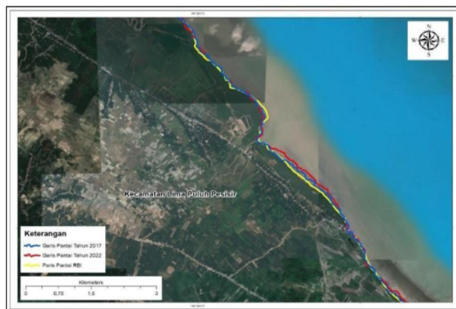
Figure 2. Results of delianiation of the Coastline of the Lima Puluh Pesisir District
