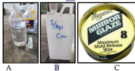
Gambar 2. A. Perekat resin poliester, B. NaOH cair, C. Wax mirror glaze
